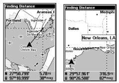
The distance from the boat's current position to the cove is 5.78 miles (left). The distance from Houston to New Orleans is 316.9 miles (right).
